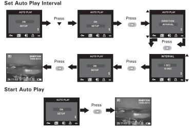
The camera will automatically run from the first file or from the last file stored. Every file will display for the specified period according to your interval setting. You can press the left or right button to manually skip backward or forward. You may press the OK button to pause or press the Wide Zoom button to stop the auto play. The auto play will keep running as long as there is power.
